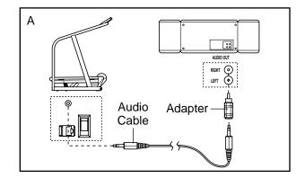
B. Plug one end of the audio cable into the jack on the side of the hiker near the power cord. Plug the other end of the cable into the LINE OUT jack on your stereo.
